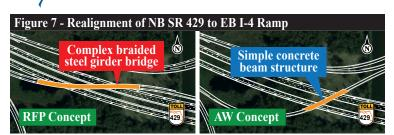
SR 417/SR 429 to I-4 EB at I-4 EB to SR 46. The AW concept "flips" this crossing from the RFP concept, placing SR 417/SR 429 to I-4 EB over I-4 EB to SR 46. This change significantly reduces retaining wall quantities, shortens schedule, and simplifies construction by keeping the ramp to SR 46 at grade (See Figure 8).
