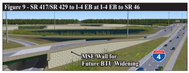
Eliminate Future Weave from I-4 EB Express Lanes to SR 417 SB with I-4 EB to SR 429 SB Exits. The weave created in the RFP Concept is completely eliminated by the AW Concept, improving traffic operations and safety (See Figure 10).
