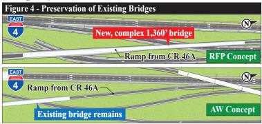
*Placement of I-4 EB Express Lane Direct Connect (Ramp EE4) over I-4 EB.* This solution, when compared to the RFP concept of running this ramp underneath I-4, provides significant enhancements:
