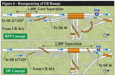
*Realignment of NB SR 429 to EB I-4 Ramp.* This allows for a more perpendicular crossing of the SR 429 mainline, replacing the complex braided steel girder bridge with a simple, concrete beam structure (See Figure 7).
