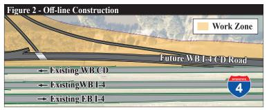
Creation of space on the eastern side of the interchange. The AW Concept also increases available room towards SR 417, allowing for improved geometry, re-use of existing structures, and elimination of bridges.
